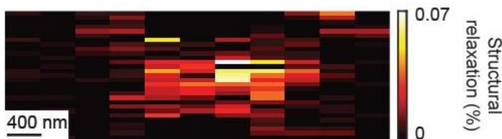
Figure 3-5: In-plane structural relaxation computed under the assumption that the strain arises only from bending of the nanoscale sheet.
