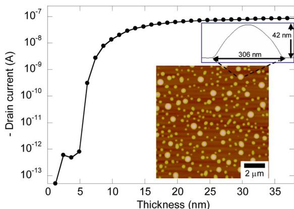
FIG. 3. (Color online) The drain current for  $V_G = -70$  V and  $V_D = -50$  V as a function of average rubrene thickness. An AFM image (inset) shows rubrene islands on the  $\text{SiO}_2/\text{Si}$  substrate with average thickness less than the percolation threshold. The sectional image shows the three-dimensional (3D) growth of a rubrene island.
