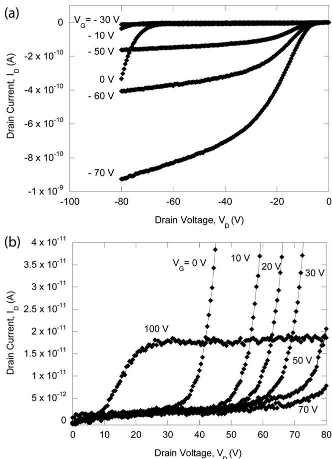
FIG. 1. Ambipolar output characteristics of a rubrene thin film transistor for (a) negative gate voltages ranging from 0 to -70 V and (b) positive gate voltages between 0 and 100 V.
