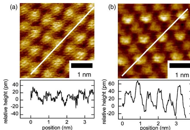
FIG. 1. (Color online) STM images of the (a) (001) and (b) (00 $\bar{1}$ ) surfaces of pentacene. A section along the highlighted line appears beneath each image.
