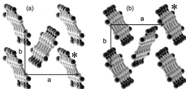
FIG. 2. Molecular models of the (a) (001) and (b) (00 $\bar{1}$ ) surfaces of a pentacene crystal based on crystallographic data from Ref. 14. The molecules closest to a central low molecule are labeled with a star.
