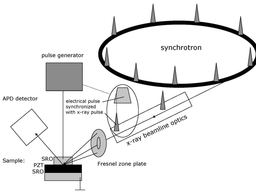
**Figure 1.** Time-resolved synchrotron x-ray microdiffraction experiment layout.
