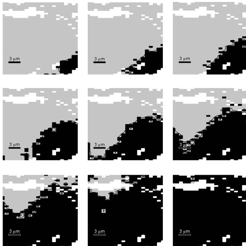
**Figure 4.** Polarization domain evolution in  $19 \times 19 \mu\text{m}^2$  sample area during 450 kV/cm electric field applied to the PZT sample. The time step between maps is 50 ns. The scale bar is 3  $\mu\text{m}$ . Gray and black areas correspond to opposite polarization directions.
