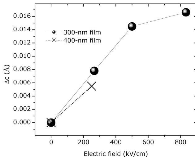
**Figure 5.** The change in the PZT *c* lattice constant as a function of the electric field.
