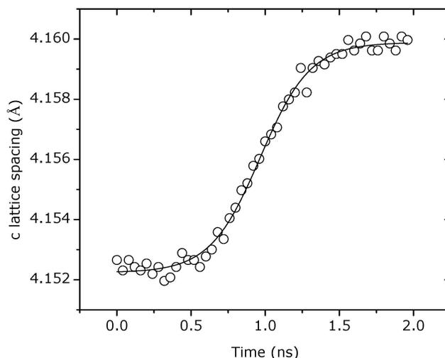
**Figure 2.** The  $c$  lattice constant of PZT as a function of time during the onset of electric field of 260 kV/cm. The 10%-90% transition time is 620 ps.
