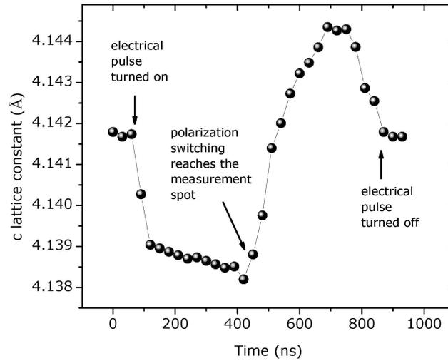
**Figure 3.** The  $c$  lattice constant as a function of time during 450 kV/cm electric field. The piezoelectric response direction changes at the time when the polarization domain wall reaches the measurement spot. The data are corrected for charging effects.
