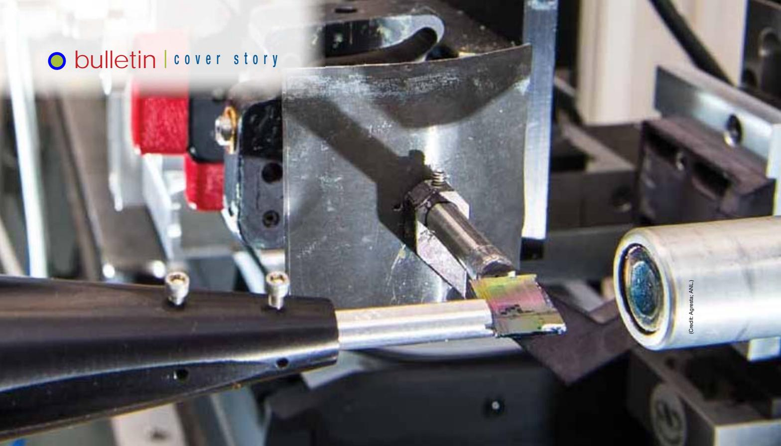
X-ray nanodiffraction instruments, such as this one at the Advanced Photon Source of Argonne National Laboratory, allow researchers to study the structure and functional properties of thin-film materials, including ceramics and the integrated circuit shown here, with spatial resolutions of tens to hundreds of nanometers.
