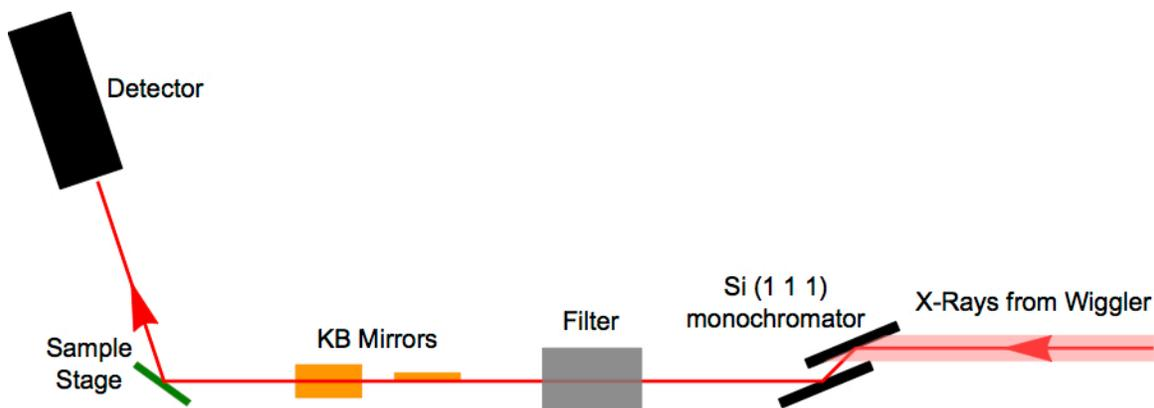
Figure 2.5 Diagram of a synchrotron x-ray beamline. The double-crystal monochromator transmits a narrow range of wavelengths. Filters attenuate the beam if necessary. A small focal spot is produced at the sample using x-ray mirrors in the Kirkpatrick-Baez (KB) geometry.
